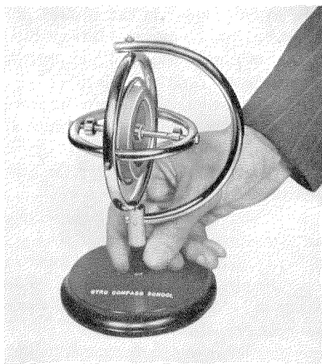
Fig. 6—When spinning, the gyro exhibits "gyroscopic inertia."
