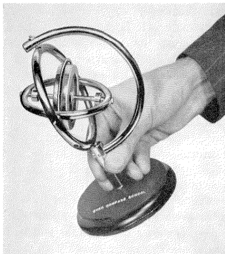
Fig. 7—The original plane of rotation is maintained no matter how the base is moved about.
